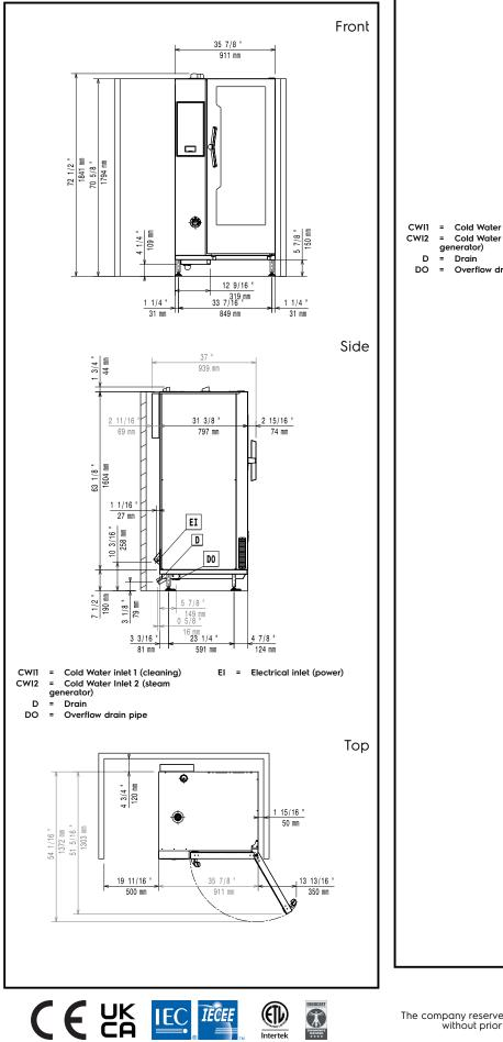
Distances CWI1 1 15/16 50 mm CW12 4 3/4 " 120 nm 15/16 EI DO D 1/16 55 mm 4 7/16 113 nr 2 Cold Water inlet 1 (cleaning) EI = Electrical inlet (power) = Cold Water Inlet 2 (steam generator) Overflow drain pipe
